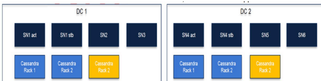
Figure 10: Cassandra with 2 racks each, where DC2 is remote, and server redundancy is used in both DCs, that is, SN1 and SN4 have standby servers. There is an extra Cassandra node in rack 2 of each DC, which could be skipped.
